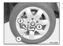
Turn adjusting screw with a screwdriver until the wheel is no longer able to turn. Then unfasten the adjusting screw 8 notches.
